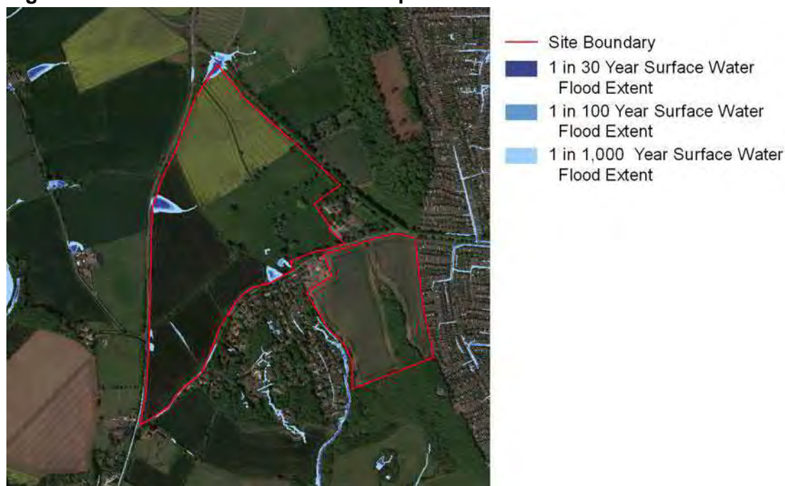
Figure 6 – Surface Water Flood Risk Map
