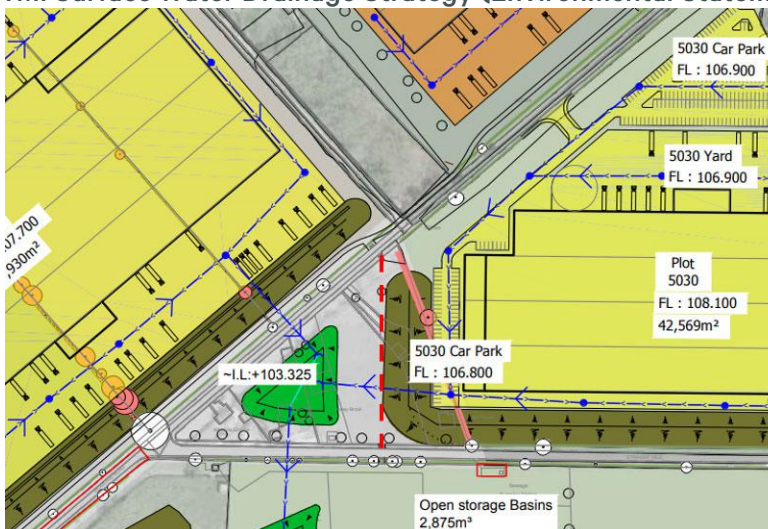
Figure 2– Draft Local Plan Green Belt boundary (red dash) superimposed approximately on approved WMI Surface Water Drainage Strategy (Environmental Statement Appendix 16.3)
