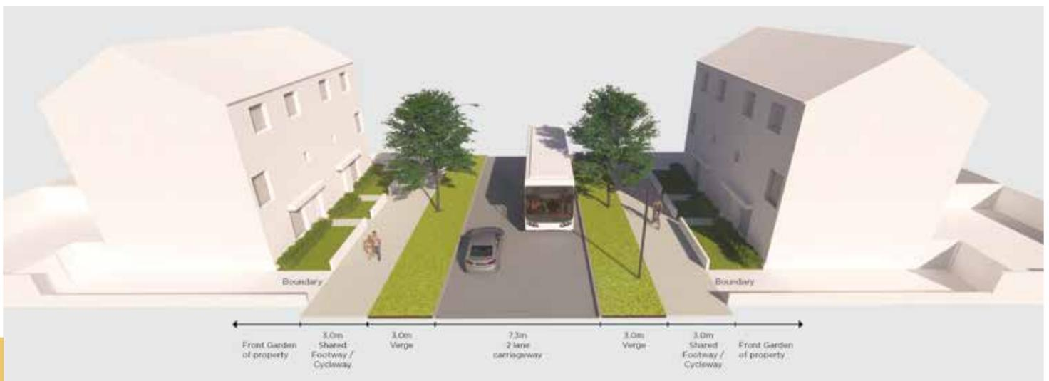
Figure 4.12 : CROSS SECTION ILLUSTRATION OF PROPOSED NEW SPINE ROAD
